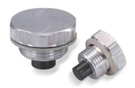
Aluminimum hex plug with a pressed-in cylindrical magnet, located in the base of the plug. This plug is fitted to the bottom of the tank, in order to collect ferrous particles that are floating in the oil, helping to protect pumps, valves and cylinders.
